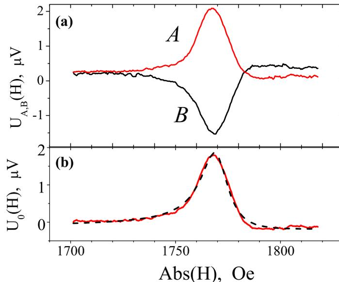
**Figure 1.** (a) The RSR voltage as recorded at opposite directions of external magnetic field  $H$ ;  $T = 308$  K,  $\alpha = 45^\circ$ ,  $P = 400$  mW. (b) The half-difference of the traces  $A$  and  $B$  (solid line) and fitting with Eq. (3) (dashed line).
