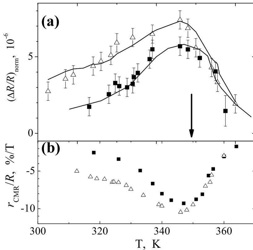
**Figure 5.** Temperature dependence of the normalized RMR magnitude (a) and differential CMR factor (b) measured on two manganite films. The curves are calculated with Eq. (5), see the text. The arrow indicates  $T_C$ .
