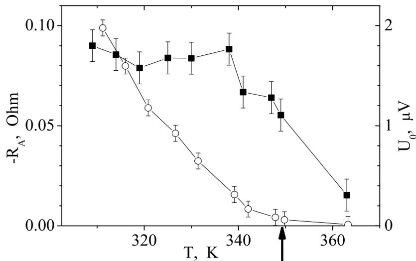
**Figure 3.** The RSR magnitude (open circles, right scale) and anisotropic part of the sample resistance (filled squares, left scale) as functions on temperature. The lines are the guides for eyes. The arrow indicates  $T_C$ .
