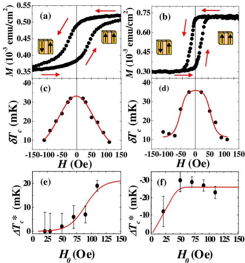
**Figure 4.** (Color online) The minor hysteresis loops for the spin valve samples with  $d_{Fe2} = 0.5 \text{ nm}$  (a) and  $d_{Fe2} = 1.3 \text{ nm}$  (b) and the dependencies of  $\delta T_c$  and  $\Delta T_c^*$  on the magnetic field value: the panels (c) and (e) correspond to the sample with  $d_{Fe2} = 0.5 \text{ nm}$  and the panels (d) and (f) correspond to the sample with  $d_{Fe2} = 1.3 \text{ nm}$  [32, 33].
