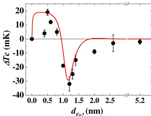
**Figure 5.** (Color online) The dependence of the  $T_c$  shift  $\Delta T_c = T_c^{\text{AP}} - T_c^{\text{P}}$  on the Fe2-layer thickness  $d_{\text{Fe2}}$ . The applied switching field  $H = \pm 110 \text{ Oe}$ . Theoretical curve (solid line) corresponds to the calculated function  $[W(0)-W(\pi)]/W(0)$  (see [38]) normalized to our experimental data [32,33]
