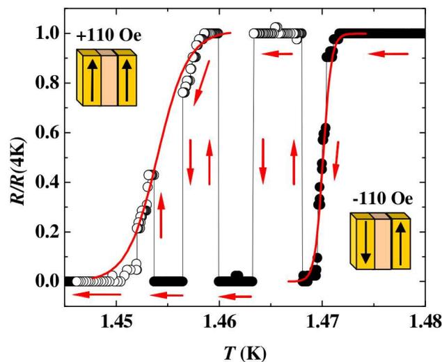
**Figure 3.** (Color online) Switching between normal and superconducting states in the spin valve sample #3 during a slow temperature sweep by applying the magnetic field  $H_0 = -110 \text{ Oe}$  (closed circles) and  $H_0 = +110 \text{ Oe}$  (open circles) in the sample plane [32,33].
