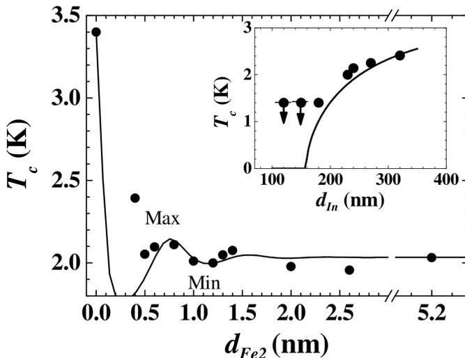
**Figure 6.** Superconducting transition temperature  $T_c$  versus the Fe2-layer thickness  $d_{\text{Fe}2}$  for the spin valve system  $\text{CoO}_x/\text{Fe}1/\text{Cu}/\text{Fe}2/\text{In}$  with a fixed thickness of the In layer  $d_{\text{In}} = 230$  nm. Inset shows the dependence of  $T_c$  on  $d_{\text{In}}$  for the set of the samples with a fixed thickness of the Fe layer  $d_{\text{Fe}2} = 3$  nm. Solid lines are theoretical fits (see the text) [33].
