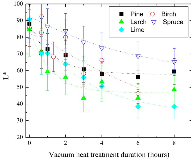
**Figure 2.** Evolution of  $L^*$  parameter values as a function of the vacuum heat treatment duration for spruce, lime, pine, birch and larch samples. The temperature of heat treatment is  $220^\circ\text{C}$ . Dotted lines represent envelope curves.
