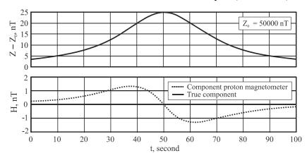
**Figure 5.** Error caused by the drift of the geomagnetic field as result of dynamic cross effect for the proton vector magnetometers (the cycle at calculations is 3 s).
