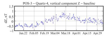
**Figure 9.** An example of long-term record of the POS-3 (Z) relative to the baseline of the theodolite DIflux magnetometer Theo-010 by taking into account variations of Quartz-4. Stability ~ 2 nT/year is. 2012.
