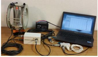
Figure 6. Vector/scalar Overhauser DNP magnetometer POS-4.
