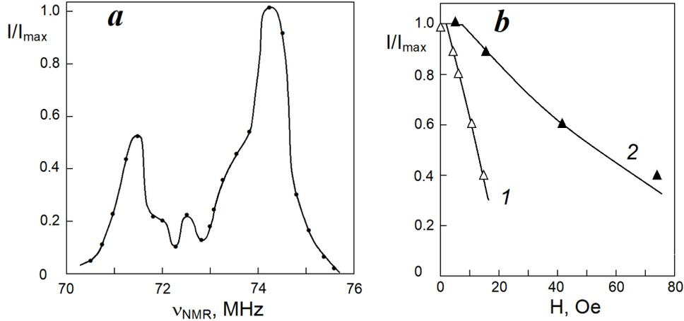
**Figure 6.** (a)  $^{57}\text{Fe}$  NMR signal spectrum in lithium-zinc ferrite; (b) Two-pulse echo (TPE) signal dependences at MVP asymmetric action on nuclei arranged in DWs in B (1) and A (2) positions. Curve 1 –  $\nu_{\text{NMR}} = 74$  MHz, Curve 2 –  $\nu_{\text{NMR}} = 71$  MHz,  $\tau_1 = \tau_2 = 1 \mu\text{s}$ ,  $\tau_d = 0.5 \mu\text{s}$ ,  $T = 77$  K.
