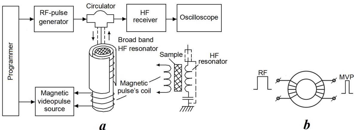
**Figure 2.** (a) Schematic of the experiment; (b) NMR cell in the case of lithium ferrite.
