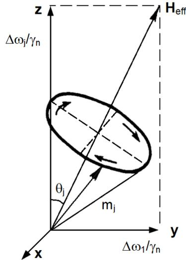
**Figure 1.** Precession of nuclear magnetization vector  $\mathbf{m}_j$  of  $j$ -th isochromate around the effective field  $\mathbf{H}_{\text{eff}}$  (1) in a rotating coordinate frame,  $\Delta\omega_j > 0$ .
