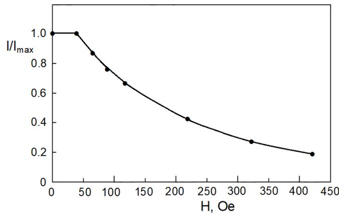
**Figure 4.** Dependences of the echo intensities on the amplitude of the magnetic videopulse in the case of cobalt micropowder,  $\nu_{\text{NMR}} = 217$  MHz,  $\tau_1 = \tau_2 = 1 \mu\text{s}$ ,  $\tau_d = 0.5 \mu\text{s}$ ,  $T = 77$  K.
