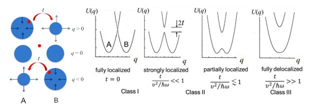
Figure 5. Illustration for the out-of-phase mode of a dimeric MV unit and its relevance to the electron transfer (left) and potential surfaces illustrating localization effect of the out-of- phase vibration in the dimeric MV unit and corresponding classification of MV (right).
