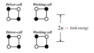
Figure 4. Schematic image of the intercell Coulomb interaction, which in the limit of strong intracell Coulomb interaction is associated with the kink energy.
