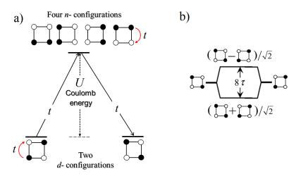
Figure 2. Schematic images of two d- and four n-configurations separated by the intracell Coulomb energy gap U and one-electron transfer processes (red arrows), which transform one of the d-configurations (left) into one of the n-configurations and then the excited n-configuration into the second d-configurations (right) (a), as well as splitting of the ground Coulomb manifold by the effective second-order electron transfer in the strong Coulomb interaction limit (b).
