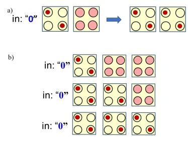
Figure 3. Illustration for the polarizing influence of the cell (input) on the neighboring cell (a) and current free transmission of information (b).
