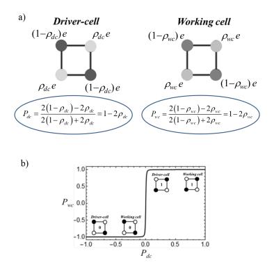
Figure 8. (a) Pair of the two-electron tetrameric square-planar QCA cells representing electric quadrupoles. Driver-cell (left part) with polarization  $P_{dc}$  acts as a source of the quadrupole field, which induces polarization  $P_{wc}$  on the working cell (right). Polarization is defined as a normalized difference between the electronic populations of the sites in one diagonal and those in another diagonal; (b) illustration for the cell-cell response function  $P_{wc}(P_{dc})$ .
