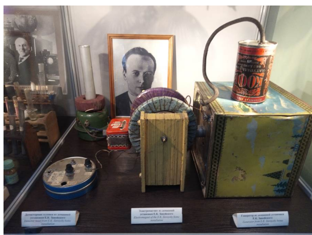
Figure 10. The Zavoisky home-made EPR setup
