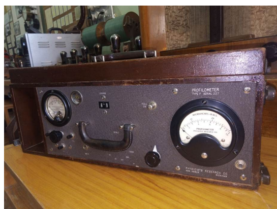
Figure 9. The American profilometer used by Zavoisky as the AC amplifier
